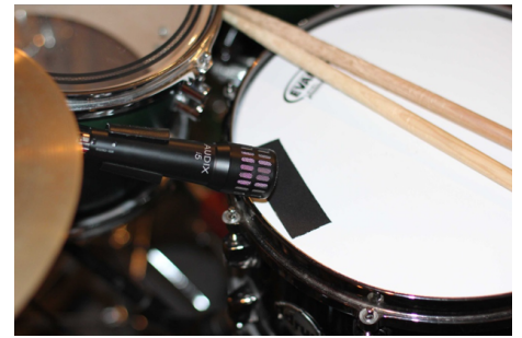
Figure 24.5: Diffuse field measurement, or close micing.
